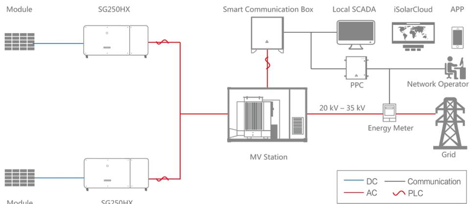
Fig.3 System Diagram
