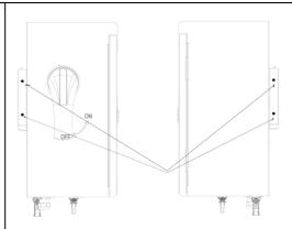
Screw from right side of wall mounting bracket
