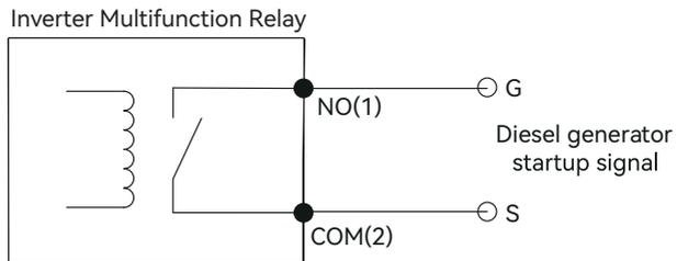
Figure 5-26 Generator Control connection diagram
