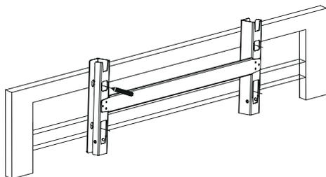
Figure 4-5 Marking hole position using installation bracket
