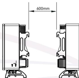
Figure 4-2C Spacing for Back to Back Installation
