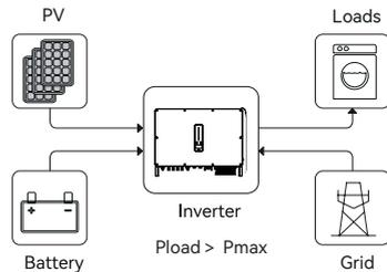
\*To realize the "Peak load Shifting" function, the load power that exceeded  $P_{max}$  has to be within the inverter max output power, otherwise, the inverter will only output the max power which allowed.
