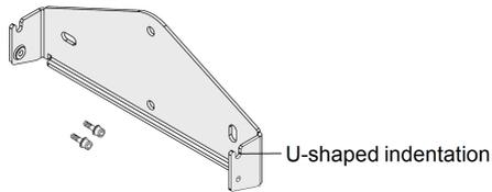
Figure 8: Mounting bracket
