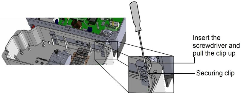
Figure 25: Disconnecting the Connection Unit from the inverter
