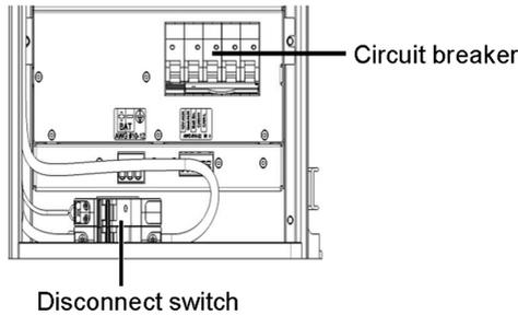
Figure 27: LG Chem battery - disconnect switch
