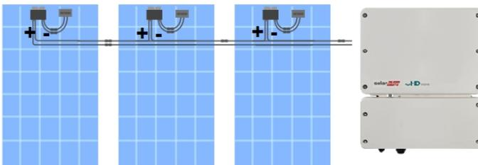
Figure 4: Power optimizers connected in series
