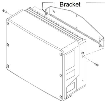
Figure 26: Mounting brackets
