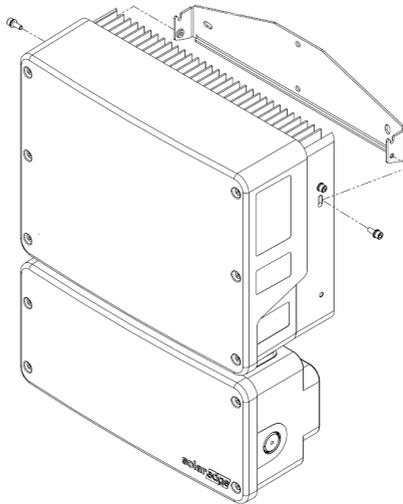
Figure 10: Hanging the inverter on the brackets
