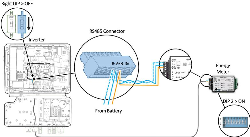
Figure 15: Meter Connection
