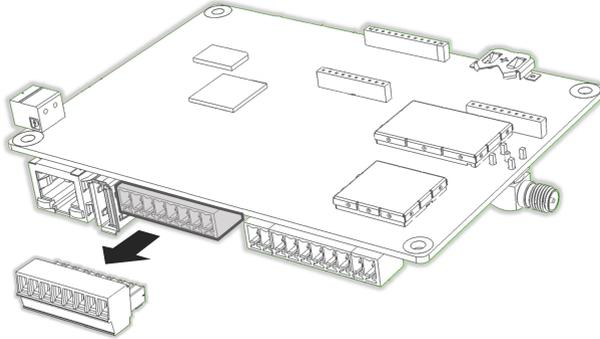
Figure 21: RS485 terminal block on the communication board
