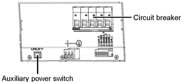
Figure 28: LG Chem battery - auxiliary switch
