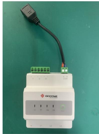
Plug the network cables from the accessory pack into the Meter port of the inverter and the port of the GM330 adapter.
