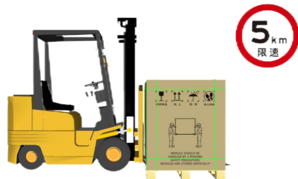
Figure 8 Note the speed of the forklift
