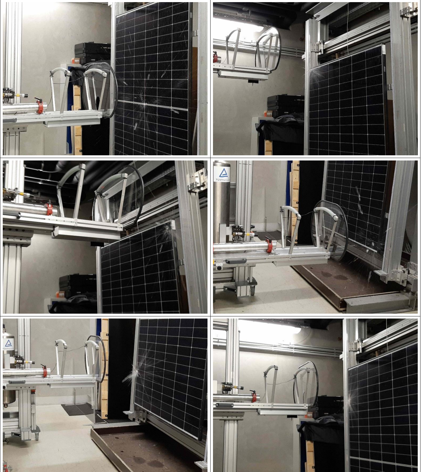
Example of Impacts on Module (30 mm)
