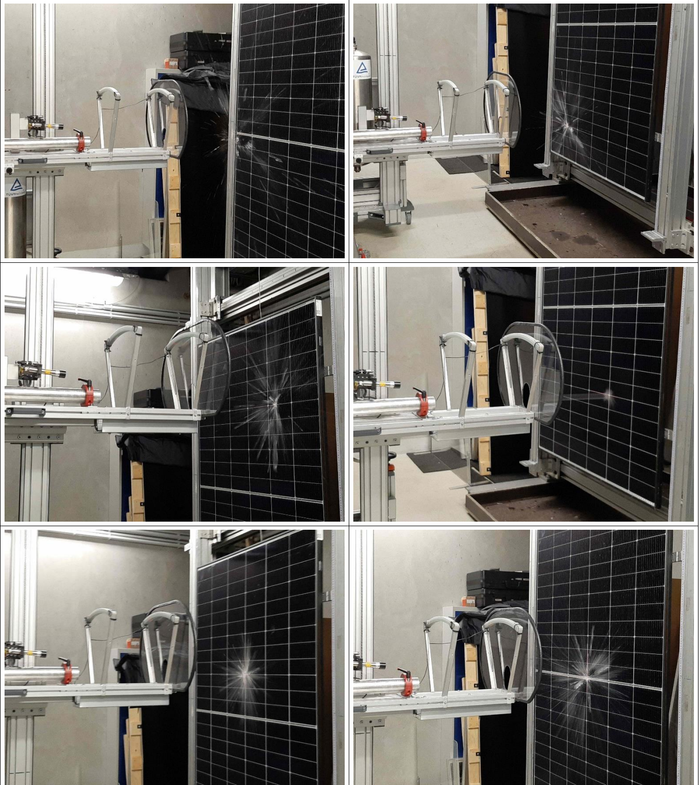
Example of Impacts on Module (30 mm)
