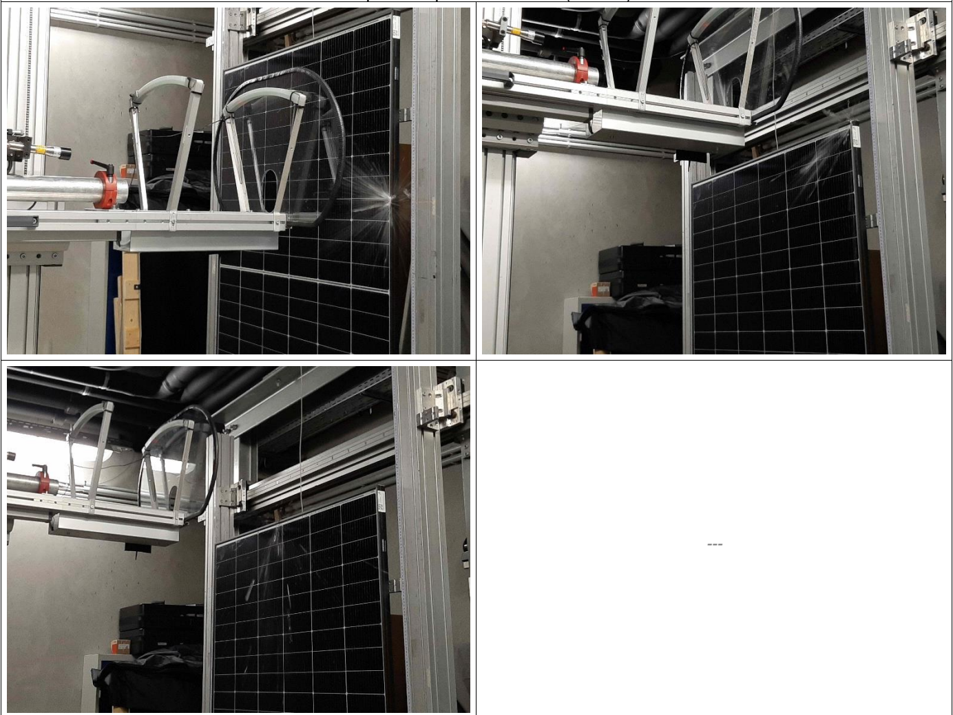
Example of Impacts on Frame (30 mm)
