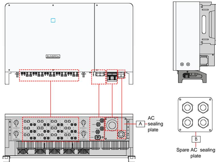
Fig.2. Wiring Terminals (Take SG250HX as an example)
