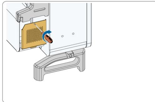
**step 3** Press the tab of the latch hook, unplug the cable connection joint outwards, and loosen the screw on the fan holder.
