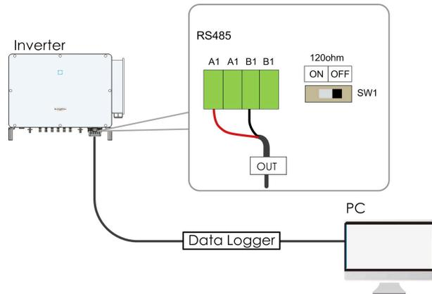
figure 5-4 Single-inverter Connection
