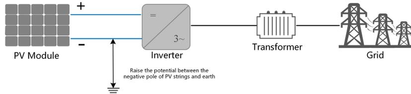
For negative voltage scheme, after the PID is enabled, the voltage to ground of all PV strings is lower than 0, and therefore the PV string-to-ground voltage is a negative value.
