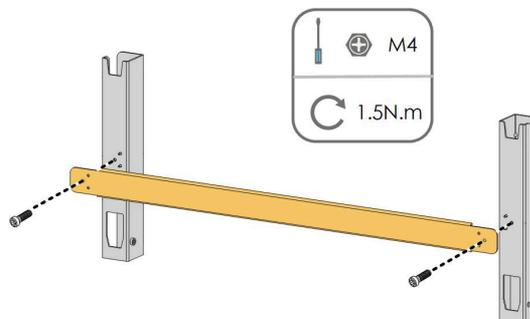
**step 2** Level the assembled mounting-bracket by using the level, and mark the positions for drilling holes.
