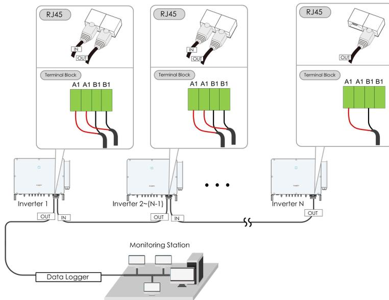
figure 5-5 Multi-inverter Connection
