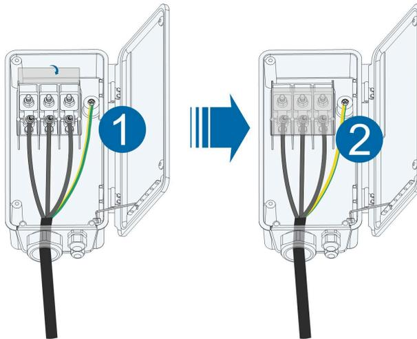
**step 11** Close the wiring compartment and tighten the two screws on its front cover with supplied Allen wrench.
