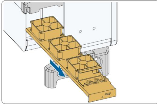
**step 5** Reinstall the fan back to the inverter in reverse order and restart the inverter.
