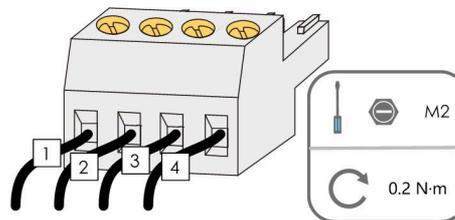
**step 5** Insert the terminal base into the corresponding terminal.
