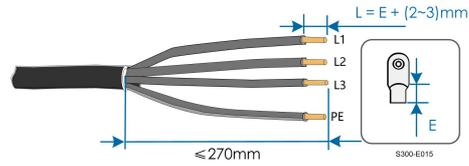
**step 8** Make the cable and crimp OT/DT terminal.
