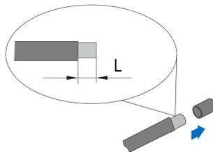
**step 2** Assemble the cable ends with the crimping pliers.
