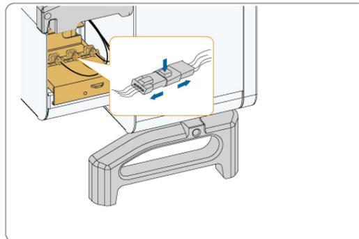
**step 4** Pull out the fan module, clean the fans with soft brush or vacuum cleaner, and replace them when necessary.
