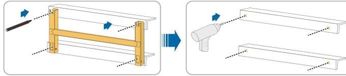
**step 3** Secure the mounting-bracket with bolts.
