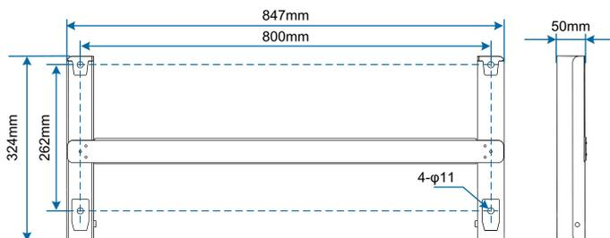
Reserve enough space when installing the mounting-bracket to meet the installation space requirements of the inverter.
