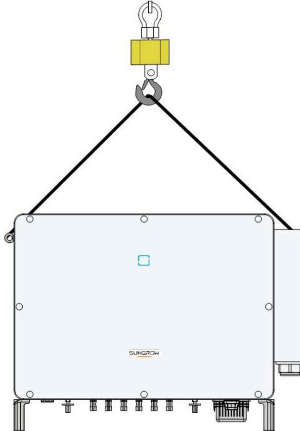
**step 4** Remove the lifting rings and reassemble the sealing screws released in Step 1.
