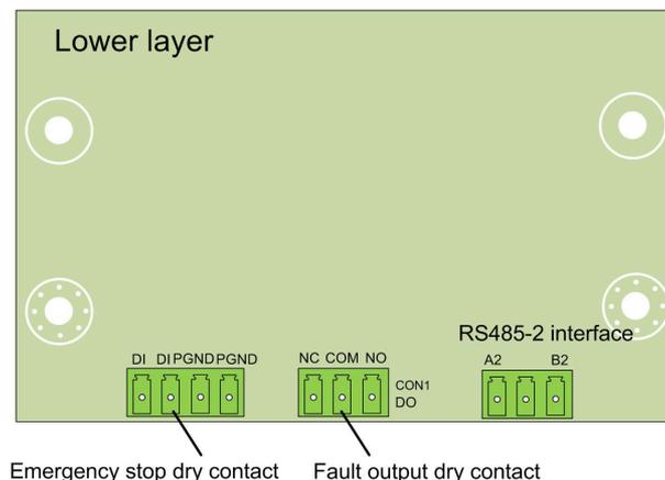
**DO terminal (fault output dry contact):** The relay can be set to output fault alarms, and user can configure it to be a normally open contact (COM & NO) or a normally closed contact (COM & NC).
