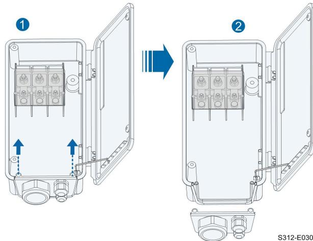
**step 4** Loosen the swivel nut of the AC waterproof connector and select a seal according to the cable outer diameter, remove the inner sealing ring if the cable diameter is larger than 40mm. Lead the cable through the swivel nut, seal, and wiring terminal successively.
