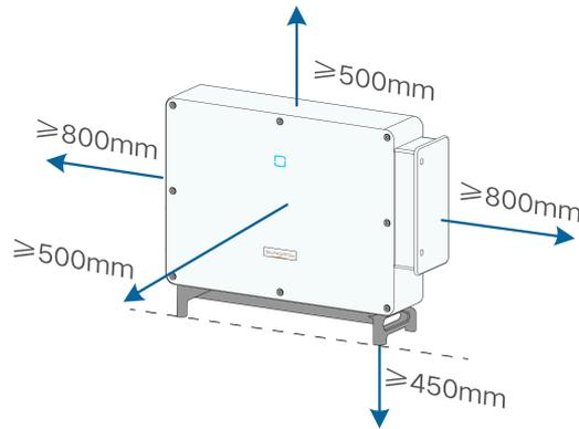
In case of multiple inverters, reserve specific clearance between the inverters.
