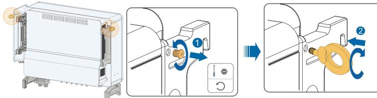
**step 2** Lead the sling through the two lifting rings and fasten the tie-down strap.
