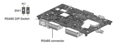
Figure 28: RS485 termination DIP-switch (SW1)
