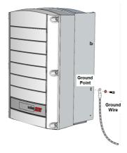
Figure 14: Grounding the Inverter
