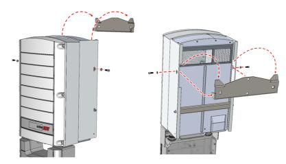
Figure 12: Hanging the inverter on the brackets
