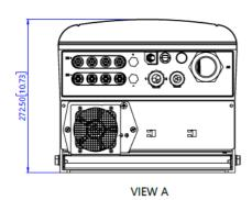
Figure 31: Dimensions of Three Phase Inverter
