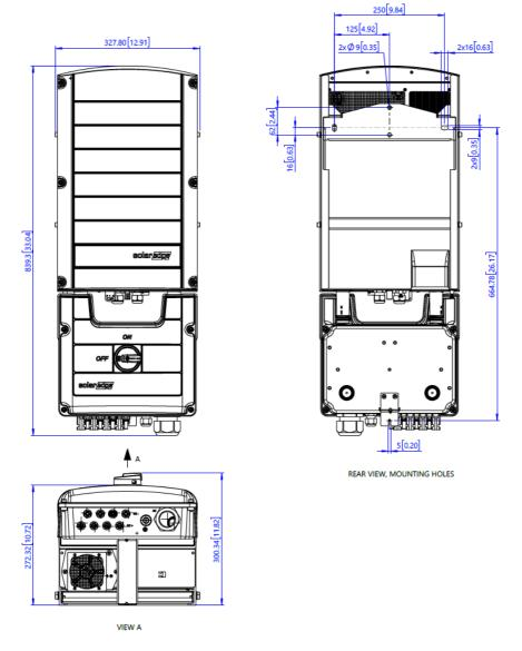
Figure 32: Dimensions of Three Phase Inverter with DC Safety Unit
