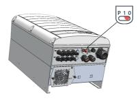
Disconnect the AC to the inverter by turning OFF the circuit breakers on the distribution panel.
