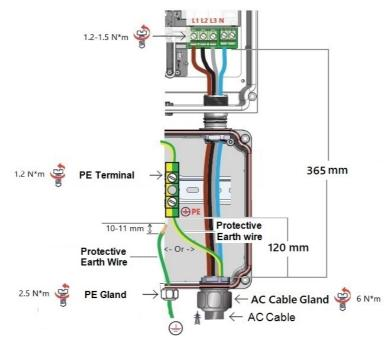
Figure 17: AC Cable and Ground Connections to Inverter with DC Safety Unit
