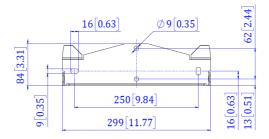
Figure 33: Dimensions of Inverter mounting bracket
