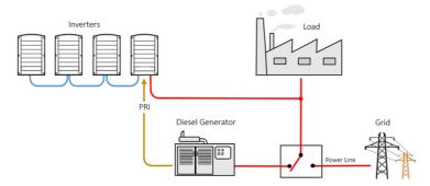
Figure 29: Example of Alternative Power Source System
