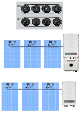
Figure 18: Inverter/DC Safety Unit DC MC4 connectors
