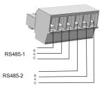
Figure 26: RS485 terminal block
