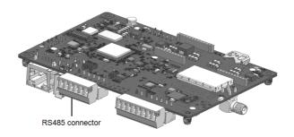
Figure 25: RS485 terminal block on the communication board
