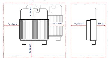
Figure 2: Power optimizer clearance
