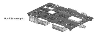
Figure 24: The RJ45 Ethernet connection
