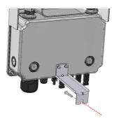
Figure 13: Securing the DC Safety Unit to the wall
