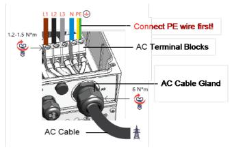
Figure 16: Connection of AC Cable to the Inverter
