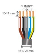
Figure 15: 5-Wire AC Cable - Insulation Stripping
