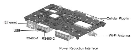
Figure 20: Internal communication connectors
