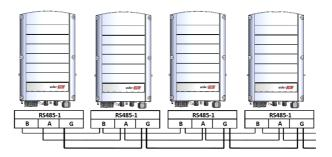
Figure 27: Connecting the inverters in chain
