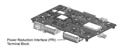
Figure 30: PRI Terminal Block Location on the Communication Board of the Inverter For detailed connection and configuration of the inverter in alternative power source mode, refer to: https://www.solaredge.com/sites/default/files/se-inverter-support-ofvoltage-sources.pdf
