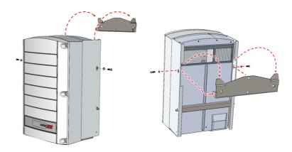
Figure 11: Hanging the inverter on the brackets
