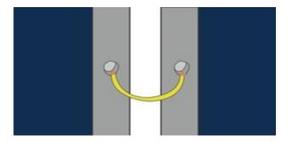
Place the toothed washers, washers, and grounding wires in turn, and screw the screws into the grounding holes to connect the two adjacent modules.
