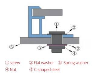
A) The mounting holes on the back of the module frame are installed on the support structure with stainless steel bolts(the screw faces the frame mounting holes)
