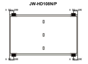
Mounted with 4 clamps along long frame. Edge Clamp: width=40-50mm, height=30mm. A=50~100mm maximum test load: front ≤1800Pa back ≤1800Pa
