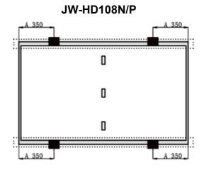
Mounted with 4 clamps along long frame. C-shaped steel parallel to the long frame. Edge Clamp: width=40-50mm, height=30mm. A=350 $\pm$ 30mm maximum test load: front  $\leq$ 2400Pa back  $\leq$ 2400Pa
