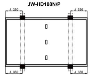
Mounted with 4 clamps along long frame. C-shaped steel perpendicular to the long frame Edge Clamp: width=40-50mm, height=30mm. A=350±30mm maximum test load: front ≤5400Pa back ≤2400Pa
