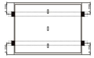
Mounted with 4 clamps along short frame. C-shaped steel parallel to the long frame. Edge Clamp: width=40-50mm, height=30mm. A=250±30mm maximum test load: front ≤4800Pa back ≤1200Pa
