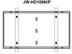
The long frame uses the inner four holes (990mm) for bolt installation
