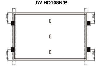
Mounted with 4 clamps along short frame. C-shaped steel parallel to the short frame. Edge Clamp: width=40-50mm, height=30mm. A=250±30mm maximum test load: front ≤1200Pa back ≤1200Pa
