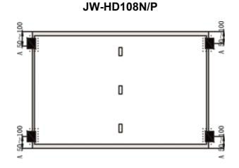
Mounted with 4 clamps along short frame. Edge Clamp: width=40-50mm, height=30mm. A=50~100mm maximum test load: front ≤1200Pa back ≤1200Pa
