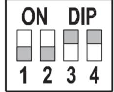
At both batteries, activate the following DIP Switches: 0010
