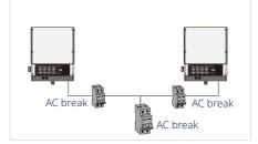
1. Use a separate AC break for individual inverter
