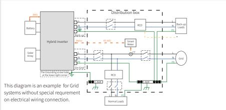
NOTE: The back-up PE line and rack earth must be grounded properly and effectively. Otherwise the back-up function may be abnormal when the grid fail.
