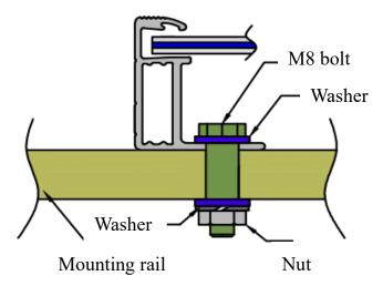
Fig. 2 Mounting with bolts
