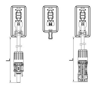
Fig. 12 (2) The half-cut cell module/ split junction box
