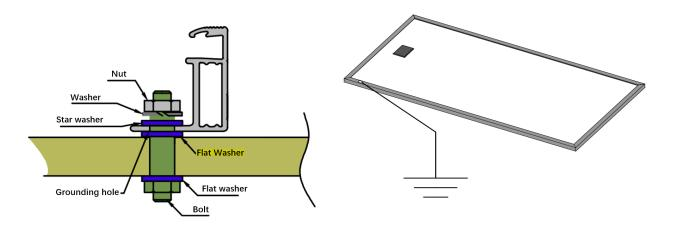
Fig. 11 Ground connection of PV modules
