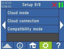
If desired, the settings of the AC ELWA 2 can also be accessed from outside the local network. For this purpose, it is necessary to register the device with serial number and device key in the my-PV Cloud: <https://live.my-pv.com/>
