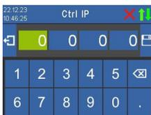
In the case of a control mode with the addition "Manual", the IP address of the signal source must not change during operation (e.g. by a DHCP router), otherwise the AC ELWA 2 will lose the control signal.
