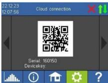
The serial number and the device key can be found under **Settings ► Cloud Connection**
