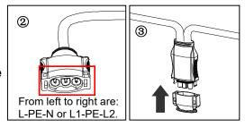
Step 7. Connect APsystems Microinverters to the PV Modules
