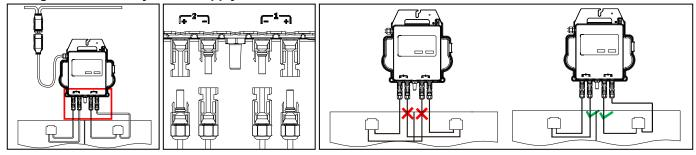
Step 8. Connect APsystems Microinverters to Grid
