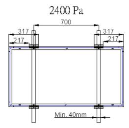
Figure 8.2 The positions of the mounted clamps
