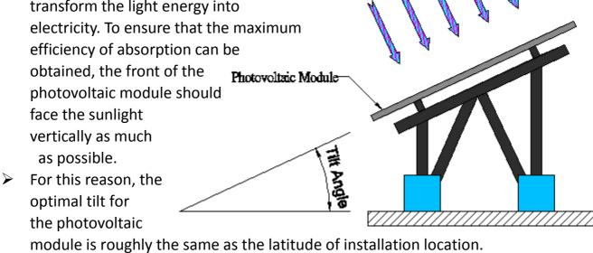
We recommend installing the modules with a tilt angle of at least 10°. To make it easier for dust to be washed off by rain and reduce the dirt or other materials that accumulate on the surface of photovoltaic modules.
