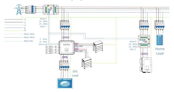
Important: Fox ESS supports the function of the second electricity meter, which is used to measure the power generation of other power generation equipment and to summarize the monitoring data on the website.
