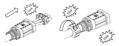
• The female end of the wire is inserted into the male end of the line and accompanied by a click sound, and the installation is complete.
