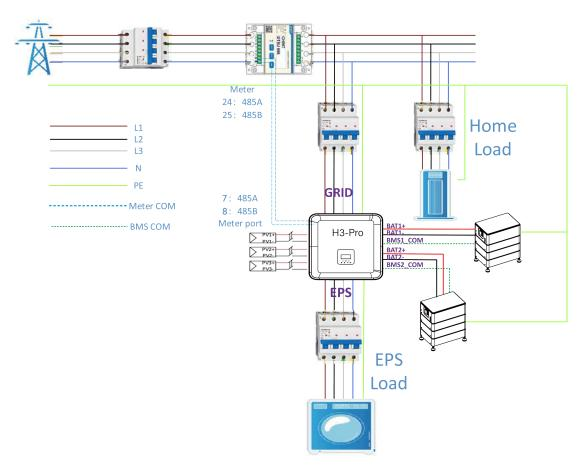
Important: H3-Pro needs to be connected to the 3-phase 5-wire power grid system, and ensure that the GRID is connected to the N line, otherwise the machine will report the SW BUS VOLT fault.
