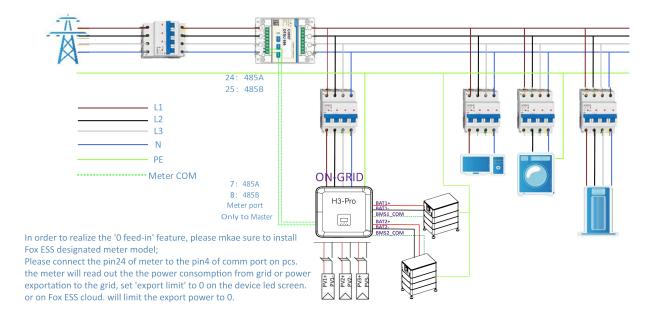
The inverter can also provide the use of two meters, using the second meter to read the power generated by another machine, where the address of the second meter is 2. When using the second meter function, you need to turn on the second meter function.
