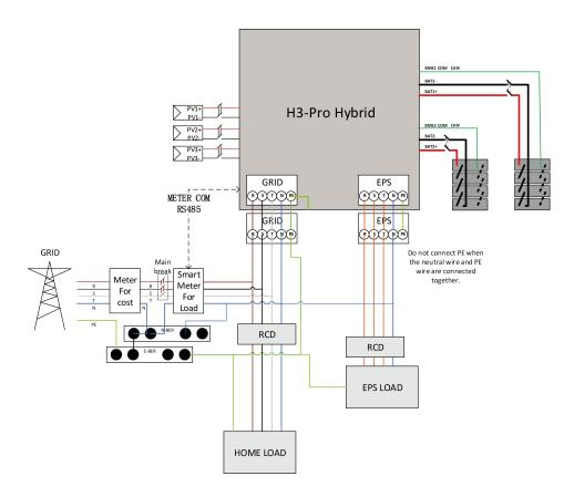
This diagram is an example for an application in which neutral is separated from the PE in the distribution box.
