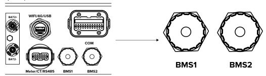
Step 2: Prepare a standard network cable and cable connector, then insert the network cable through the cable connector.
