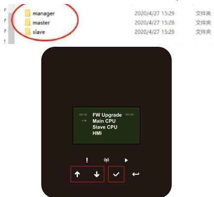
6. Remove the USB disk after upgrade completed. Follow the procedure blew and click the option to view the version:
