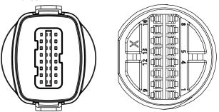
METER/CT/RS485 interface (20pin terminals)
