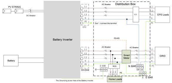
For countries such as China, Germany, the Czech Republic, Italy, etc, please follow local wiring regulations. This diagram is an example for an application in which neutral is separated from the PE in the distribution box.
