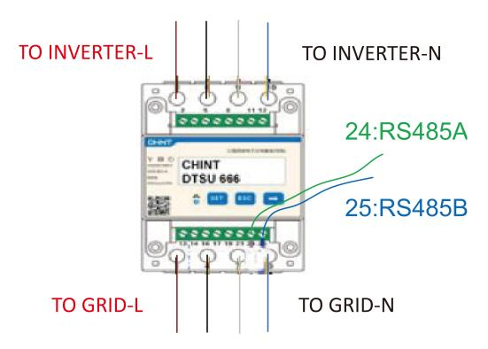
Insert L1/L2/L3/N wires and RS485A/B cable into the meter.Please refer to the meter wiring diagram on side of meter itself.
