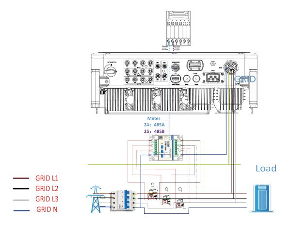
Insert L1/L2/L3/N wires ,CT and RS485A/B cable into the meter.Please refer to the meter wiring diagram on side of meter itself.
