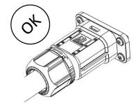
Use a screwdriver to align the unlock position and press and Hold the thread and pull it back to complete the separation of the male and female.
