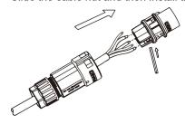
• Push the threaded sleeve into the socket, tighten up the cap on the terminal and the torque is (4-5N.m).
