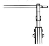
• Insert pin contact through the cable nut to assemble into back of the male or female plug. When you feel or hear a "click" the pin contact assembly is seated correctly.
