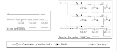
If the module is passed through by a reverse current greater than the maximum fuse current of the module, the module shall be protected with an over current protector of the same specification. If more than two strings are connected in parallel, each module string shall be protected with an over current protector as shown above.
