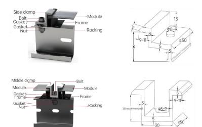
Under no circumstances should the clamp touch the glass or deform the frame. Be sure to avoid shadowing effect from the pressure clamp.
