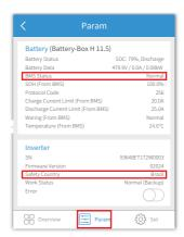
Note: For compatible lithium batteries, the BMS status will display "Normal" after selecting the correct battery company.
