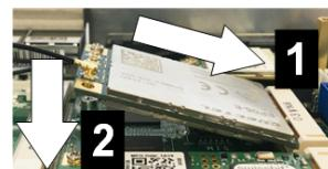
Fig. 5-10: Inserting the circuit board
